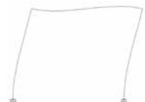
Fig 2: Deflected shape at mechanism level
