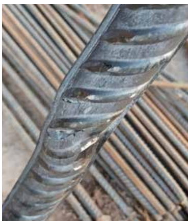
Fig 1: Bend and Rebend test for Reinforcing bars
